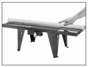
**Figure 6.** Using a straightedge to ensure the working surfaces are flush.
